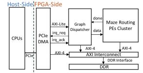
Fig. 2: The FPGA Acceleration Framework on AWS Elastic Compute Cloud (EC2) [11].
