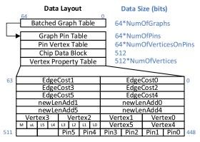
Fig. 1: Data Layout in FPGA Memory.
