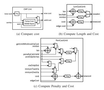
Fig. 7: Computing Units in PPU and PCU.
