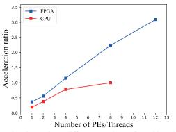
Fig. 9: Acceleration ratio at different numbers of PEs/threads (batch size = 5923).
