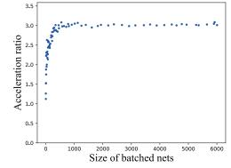
Fig. 8: Acceleration ratio at different batch size compared with 8-thread CPU.
