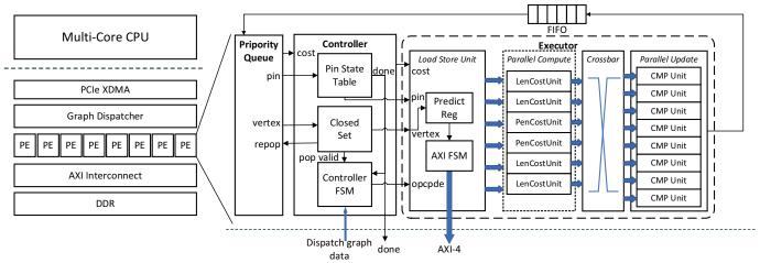
Fig. 3: Structure of Maze Routing Processing Element.
