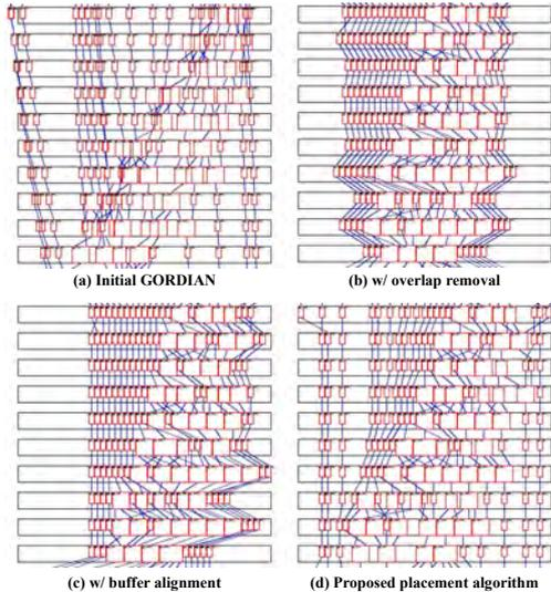
Fig. 4: The example comparison placement diagrams of an 8-bit Kogge-Stone adder (partial circuit).
