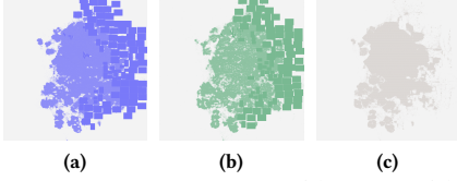
Figure 7: 3D placement of bp_quad: (a) top die, (b) bottom die, and (c) HBT layout of our timing-driven placer.
