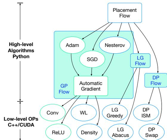
Figure 1: Software architecture of DREAMPlace [10].
