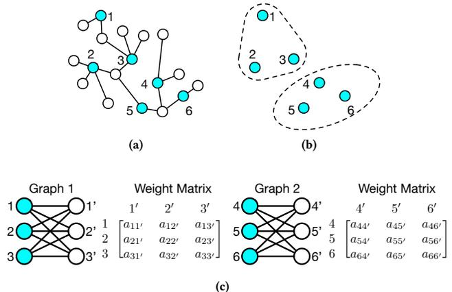
Figure 2: Steps for batch-based independent set matching [13]. (a) Maximal independent set extraction. (b) Independent set partitioning. (c) Batched bipartite matching.
