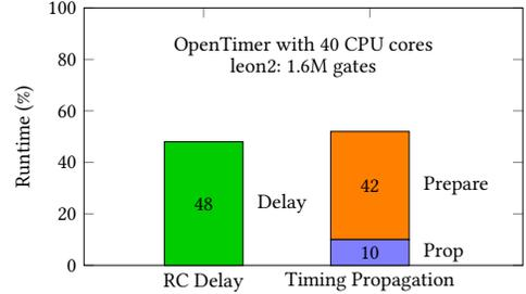
Figure 4: Runtime breakdown for OpenTimer to compute full timing on a million-gate circuit using 40 CPUs [23].
