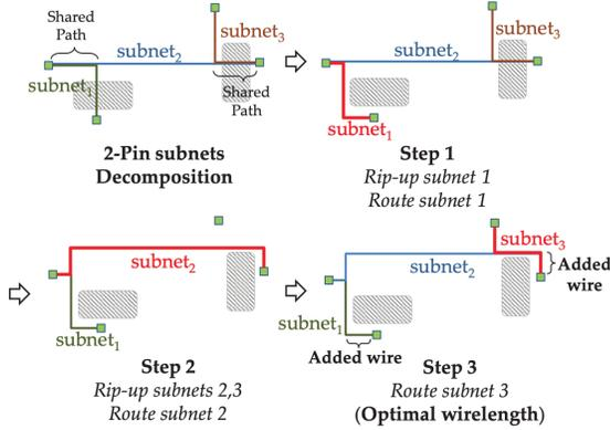
Figure 3: Net decomposition to increase the parallelism [19].
