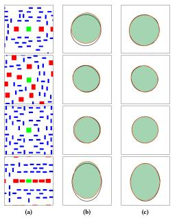
Figure 6: (a) Mask pattern input (b) CGAN output and (c) LithoGAN output. Each row represents one clip example. The golden contour is outlined in black. The prediction pattern is filled with green and outlined in red.
