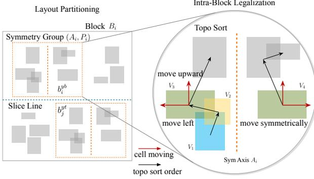
Fig. 4: Layout partitioning and intra-block legalization.
