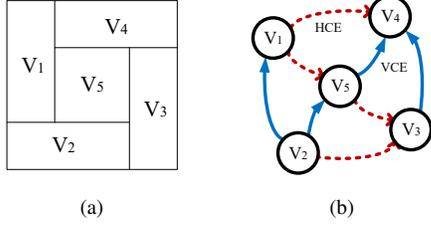
Fig. 3: Mixed constraint graph with horizontal constraint edges (HCEs) and vertical constraint edges (VCEs).
