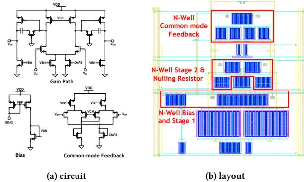
Figure 1: Op-amp circuit and layout example.
