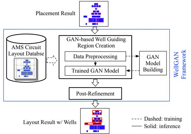
Figure 3: Proposed well generation framework (WellGAN). certain value. Finally, the minimum area rules suggest the enclosing area of the well should be no less than a certain value.
