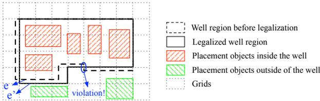
Figure 8: Grid-based method for the minimum width rule.
