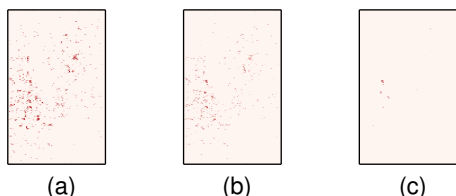
Fig. 5: The EM violation map of design leon2 . The tiles with violations are marked in red. (a) The initial design, (b) after single row placement, and (c) after single tile placement.
